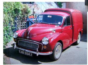
Kustom Kolors I started to re-assemble the van. I upgraded the brake system to disc brakes and servo and fitted  $5^{1}/_{2}J$  steel wheels. It took approximately 11 months to finish my latest project and have it MOT'd and on the road.
