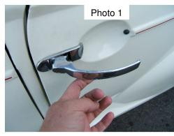
Do you have droopy door handles? It seems to be a common fault on the Minor – particularly on the 4-door models (probably due to it having twice as many doors!). The return spring which holds the chromed handle against the small black buffer often gives up and leaves the handle to rattle around unrestrained. This is not a 'show stopper' since it doesn't affect the operation of the door itself, but it is a nuisance and it may annoy some owners (OK, just me then!). The cure is to take
