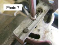
head holds the spring in place. Approximately 3mm length seems to work and a hole diameter of 2.5mm was used. I have successfully done this on two cars now and it seems to work. (Editor) Good luck.
