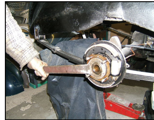
Eddie tightens the hub nuts with yet another home made 'BMC Service Tool'
