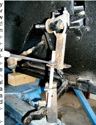
Surrogate steering leg being tightened prior to fitting stub axle and trunnions.
