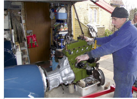
Eddie – hoisting the engine and gearbox into place
