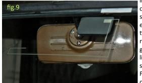
inside of the windscreen. The cable can be tucked behind the windscreen rubber, emerging at the lower corner and the aerial itself is partially hidden by the rear view mirror. That shown in fig.8 has an integral signal amplifier which requires a live connection - to one of those spare blue wires mentioned earlier. Fig. 9 shows an internal aerial for digital signals.
