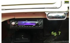
There are either one or two more power related wires attached to the modern radios; one blue, the other blue/white. One for electric aerial operation, the other to power an auxiliary amplifier. They will be redundant in most Minor installations but both become live when the radio is switched on, so precaution should be taken to ensure that
