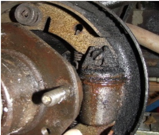
Fig.1 Typical view of leaking front cylinder. (Note Non-standard beehive spring—not really necessary!)
