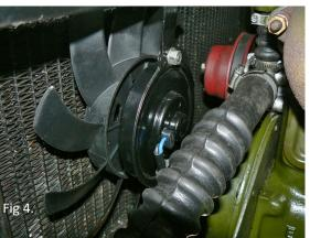
ed if the reader is prepared to splash out on a ready-made 'kit'. Some kits are designed to have the fan mounted behind the radiator, sucking the air through. Other kits such as seen in figs. 2 & 3 include fans which are quite slim and can be operated as a 'blower', being discretely fitted in between the grille and the radiator on a Minor. A depth of 2" should be considered the maximum for front-fitting.
