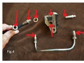
parts which are to be fitted have been cleaned, inspected and replaced where necessary, reassembly can commence, and will be dealt with next month. Pass the hose through the front slot of the backplate, place the washer over the free end of the flexible hose and screw the upper hole of the cylinder
