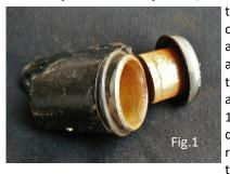
that are not used frequently. The wheel cylinders of the Minor suffer the same two basic problems as any other vehicle's wheel cylinders, leaking and seizing. Their design leaves every opportunity for dampness to instigate corrosion and a small amount of corrosion leads quickly to seizure. Fig. 1 shows the rust formed after a short lay-up in damp conditions. Once piston and cylinder have rusted together it is almost impossible to free them without causing damage. If your car is laid
