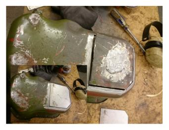
Whilst re-assembling the engine for my convertible, I noticed what appeared to be rather untidy bit of brazing inside the sump. Further investigation revealed an equally untidy blob of body solder on the outside. I then spent best part of a morning, making and fitting a replacement piece which was welded top and bottom, tested for leaks overnight with paraffin and found to be OK.
