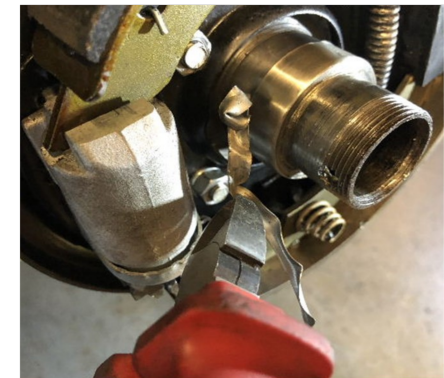
Collar being torn off with side cutters showing Showing finished article—ready for reassembly .
