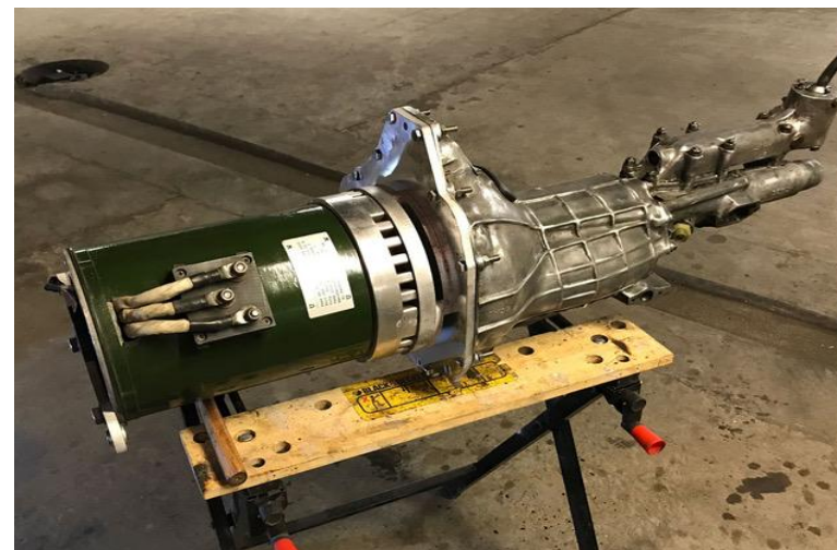
The 'A' Series gearbox with purpose made adaptor plates. (In this Instance connected to a new HPEVS-31 Motor)
