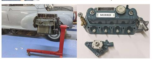
The sump cover, crank pulley, stater dog, front and rear panels were all taken back to bare metal after using paint stripper and a wire wheel brush. Then applying Kurust, VHT primer and \* Pru Blue (\*an original colour) HT enamel paint. These all look nice and are ready to go back onto the block when it is back with me.
