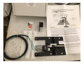
This is a kit which overcomes the inherent problem of the weakness in the conventional hydraulic brake light switch fitted to the Minor. This switch kit works in parallel to the original switch which can be left in place and utilises a micro-switch and relay to operate the brake lights as soon as the pedal is touched. This increases safety as the lights are illuminated sooner and are not subject to the common problem of arcing and burning-out of the existing switch under the radiator.
