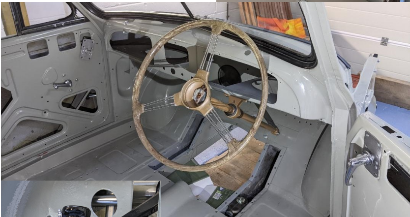
The refurbished steering rack and steering column and one of several steering wheels are now fitted.
