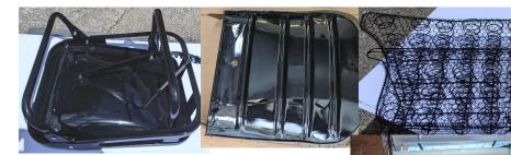
I had restored the front seat frames, shot blasting and zinc plating and spraying them gloss black. The back seat squab and back rest were stripped back to the frames and springs which I applied Kurust to and gloss black sprayed. I used 7 cans of paint on the base frame and springs as most of the paint went straight through.
