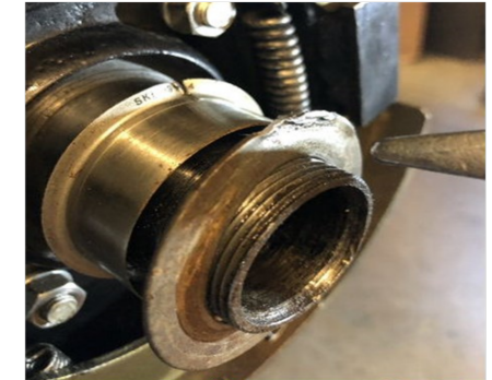
Sleeve on other side being fitted using an old locking Washer to gently ease it over the axle.
