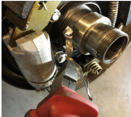
Collar being torn off with side cutters showing Showing finished article—ready for reassembly .
