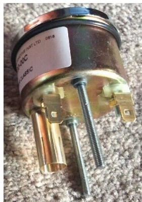
Rear of a 'new spares' voltmeter
