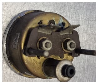
Rear of the original Smiths ammeter
