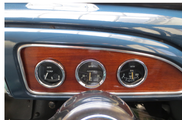
Editors saloon 'D.I.Y.' glove box panel Smiths Water temp - Ammeter - Oil pressure
