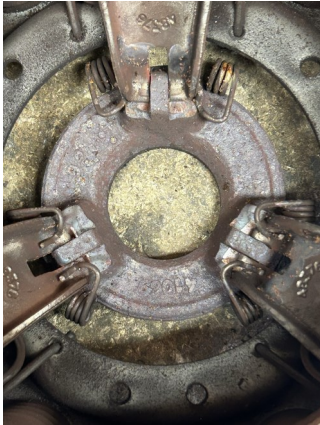
This shows the inner release ring assembly with the three retaining springs fitted but with the top one dislodged on both sides (viewed from inside the clutch)
