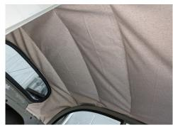
bought from ESM a year ago. I recently fitted the 4 hooped roof supports into the new lining and stitched the material to tighten to the ends of the hoops. I followed Newtons guide which gave exact measurements to attach the plywood panel to the material to then insert over into the front cant rail above the screen. In it went but the
